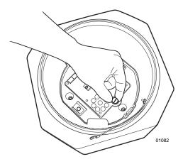
a. Turn the thumbscrew and open the hinged door located inside the back box.
